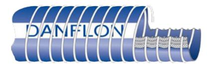
Used Worldwide by many leading companies, these premium quality hoses are lined, as standard, with Ethylene Chloro Tri Fluoro Ethylene (ECTFE). This is a high tech fluropolymer very similar to Poly Tetra Fluoro Ethylene (PTFE) in its broad spectrum chemical resistance but with the advantage of high mechanical strength and low permeability. The inner and outer wires can be galvanised carbon steel or stainless steel 316.
